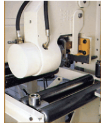
Punching unit of 50 t. for vertical leg of the angle with simple punch up to Ø 31 mm.
